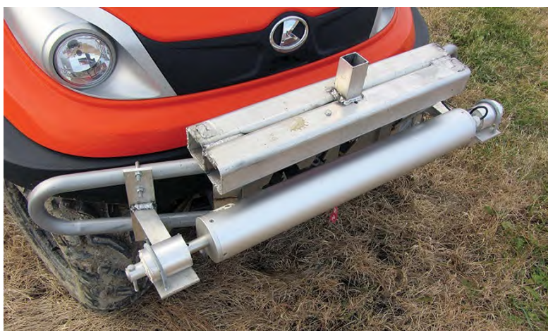
A vehicle-mounted passive gamma-ray sensor.
